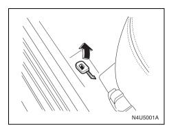
To open the fuel filler door, pull up on the fuel filler door release lever located on the floor to the left of the driver's seat.
